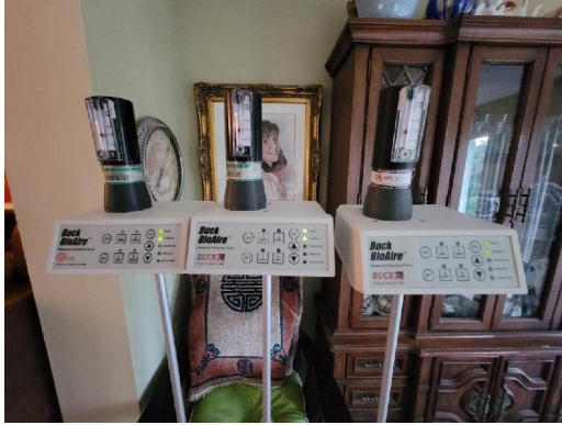
Pumps B153637, B153638, B154503 Calibration prior to testing
